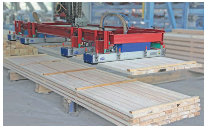
Wood | Vacuum suction spider SSP on an industrial gantry for handling rough sawn wooden boards
