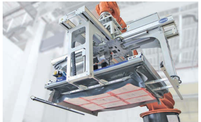
Intra logistics | Vacuum layer gripping system SPZ-M-C for the handling of various product layers in department store and intra logistics
