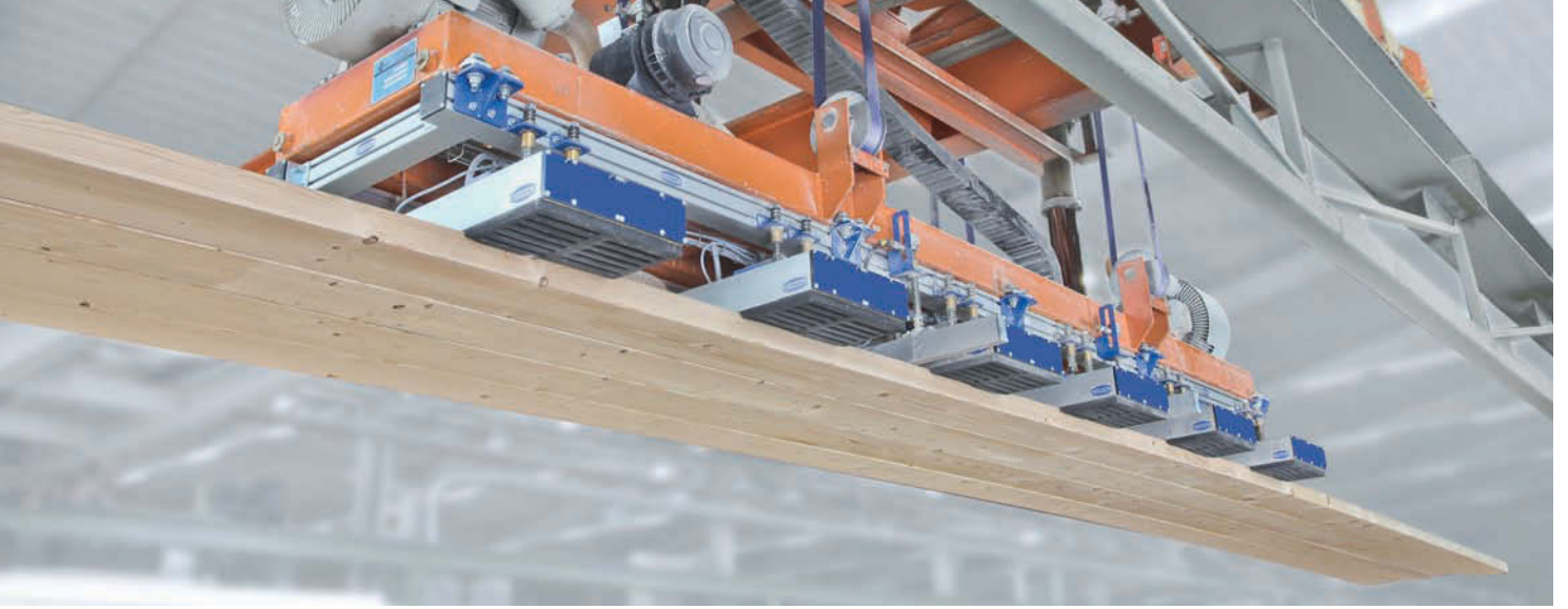
Vacuum suction spider SSP for the layered stacking of wooden boards for the construction of prefabricated houses
