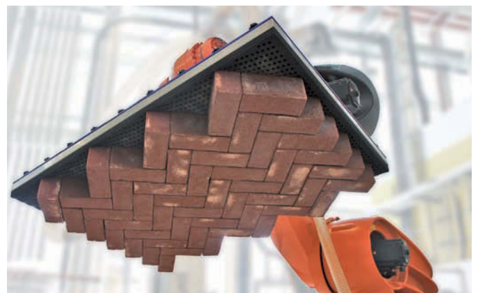
Construction materials | Vacuum layer gripping system SPZ for the handling of clinker bricks
