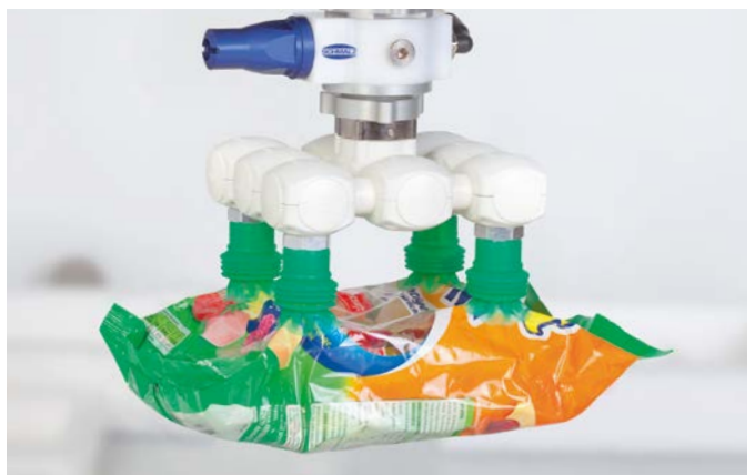
Vacuum end effector with bellows suction cups SPB4f handling pouches
